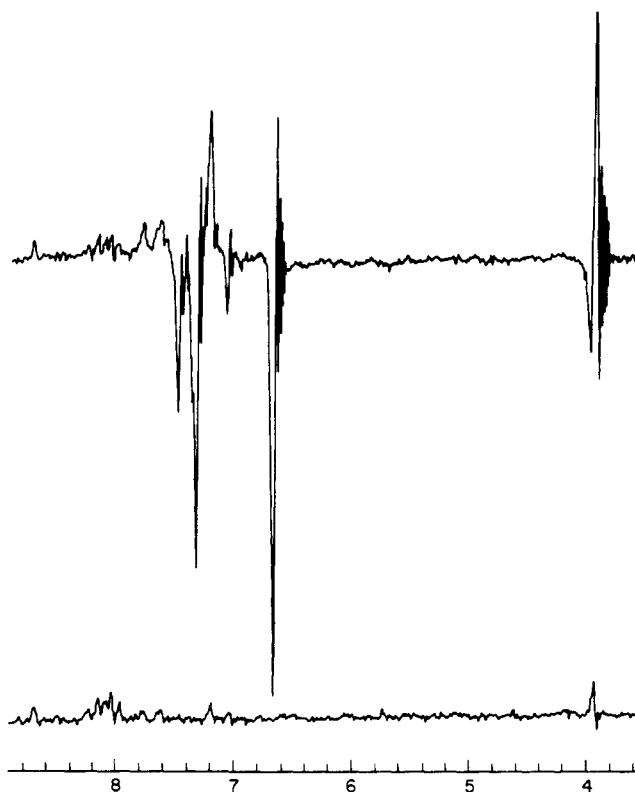
Figure 4. 60-MHz ^1\text{H} NMR spectra observed during the irradiation of 9-cyanophenanthrene (0.02 M) in the presence of trans -dimethoxystilbene ( \sim 0.005\text{M} ) in acetonitrile- d_3 (top) and in the dark (bottom).
